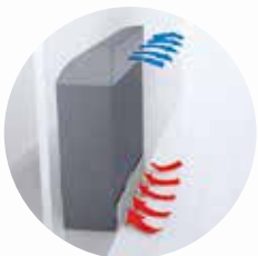
Airflow: OVER, air discharged from the top, air intake from the rear/bottom of the unit
